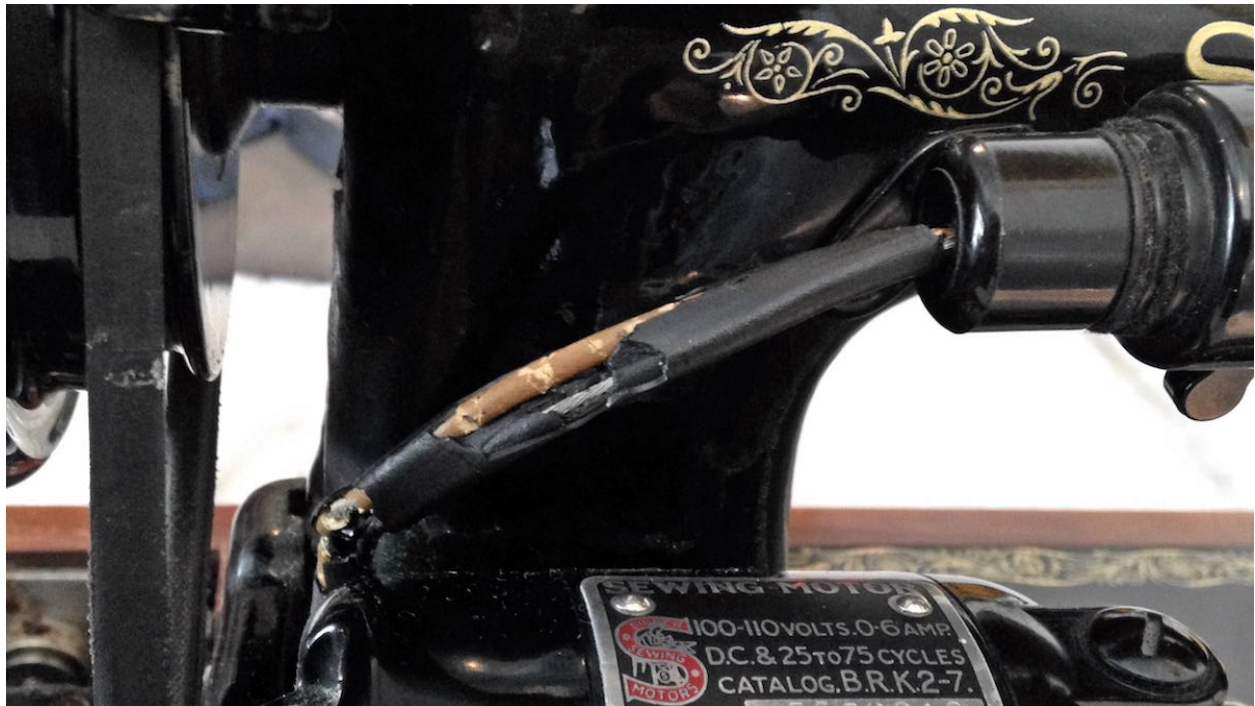
Damaged Wiring on the SINGER® 99K
